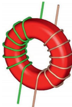
**Sectional winding:** Shows the highest attenuation in differential mode. These chokes are recommended for power lines, where a high isolation is mandatory and the power delivery is happening at low frequency.
