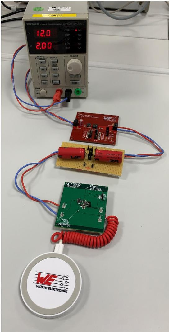
**Figure 9: Picture of the complete application with the different power converter, Supercapacitor bank and the load but with a different power supply.**
