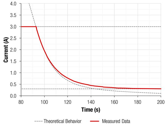
**Figure 7: Charging Current with off-set current of 0.3 A.**
