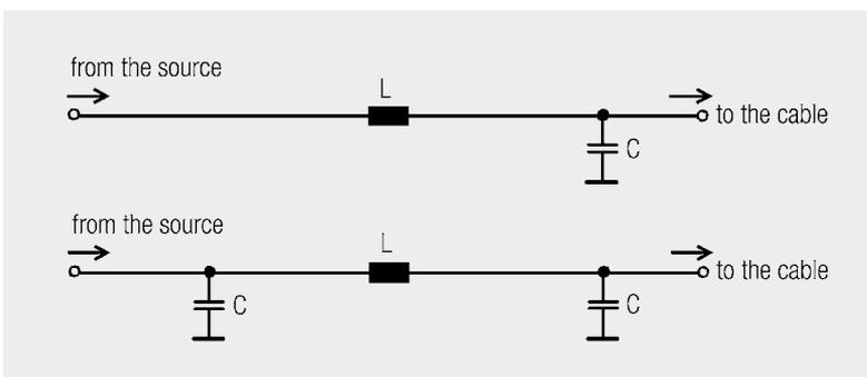
Fig. 3.6: Interface filter circuit versions (common-mode versions not considered)
