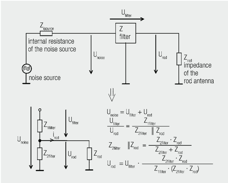
Fig. 3.5: Impedance relationships at the peripheral cable interface
