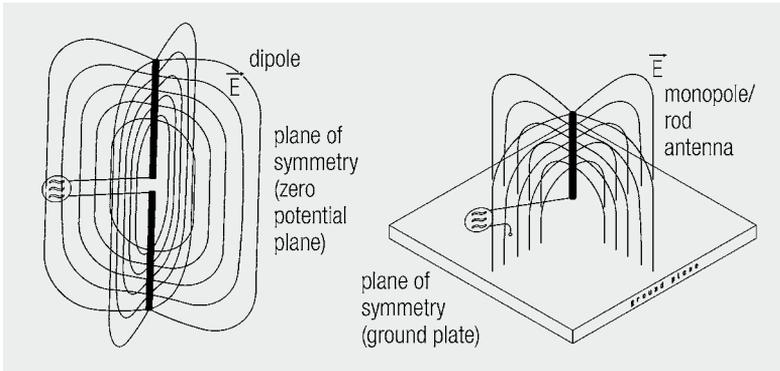
Fig. 3.2: Conversion of the symmetrical dipole to a rod antenna
