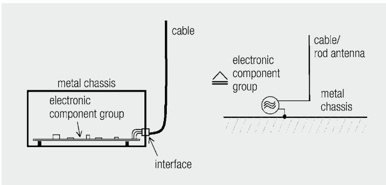
Fig. 3.3: Relationship between peripheral cable and rod antenna
