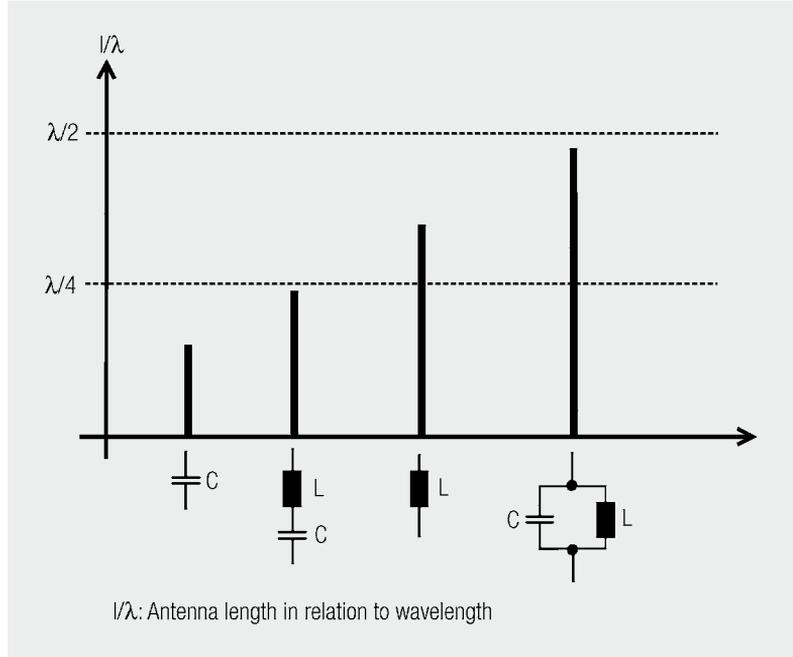
Fig. 3.4: Equivalent circuit of the rod antenna is dependent on the antenna length
