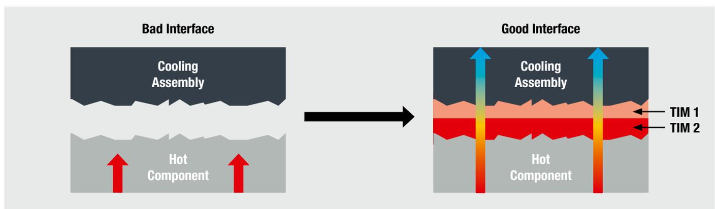
**Fig. 3:** Detail of contact surfaces
