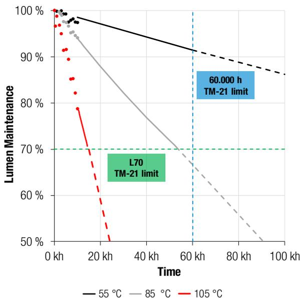
**Figure 7: Typical Lumen Maintenance of One Type of LED at Different Operating Temperatures [13]. Markers Represent Measured Data and Lines the extrapolated Lifespan as per IES TM-21. Dashed Lines Represent Predictions Beyond the Limits of TM-21**
