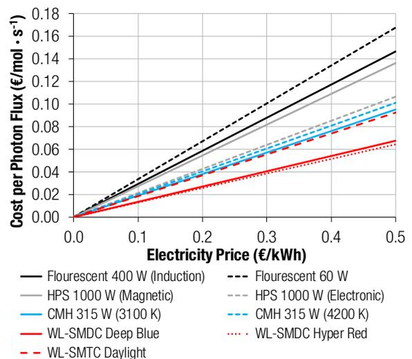
Figure 4: Cost per PPF as a Function of Electricity Prices in High-Pressure Sodium (Grey), Metal Halide (Blue), Fluorescent (Black) and LED (Red).
