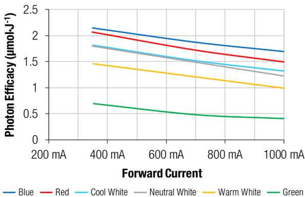
Figure 3: Typical Photon Efficiency ( $\mu\text{mol}/\text{J}$ ) as a Function of Input Forward Current (mA)
