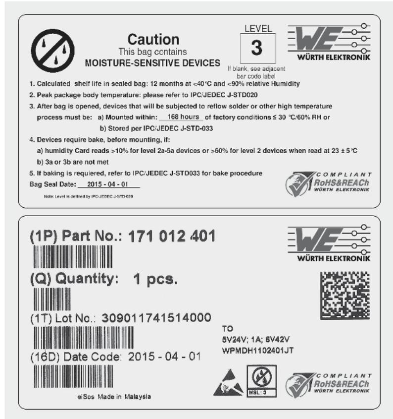
Fig. 5.1: Example: bag label for power module article no.: 171 012 401
