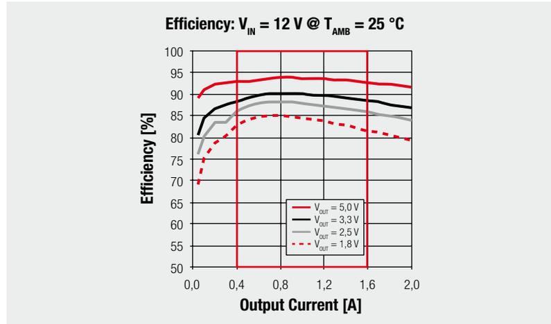
Fig. 6.2: Efficiency taking the example of order code 171020601
