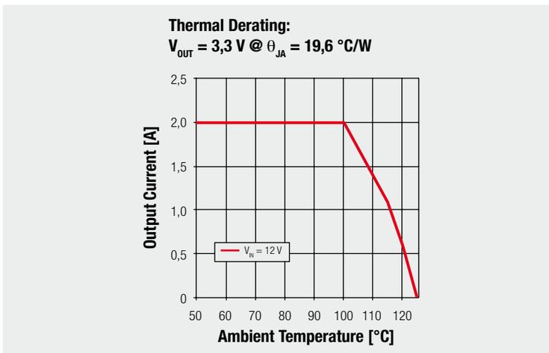
Fig. 6.1: Thermal derating taking the example of order code 171020601
