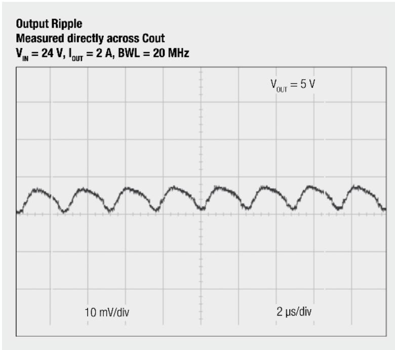
Fig. 6.3: Output voltage ripple @ 5 V taking the example of order code 171020601
